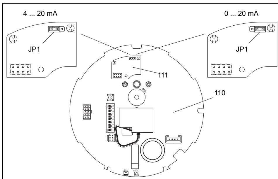
**diagram 13** Set signal range for mA output signal X
