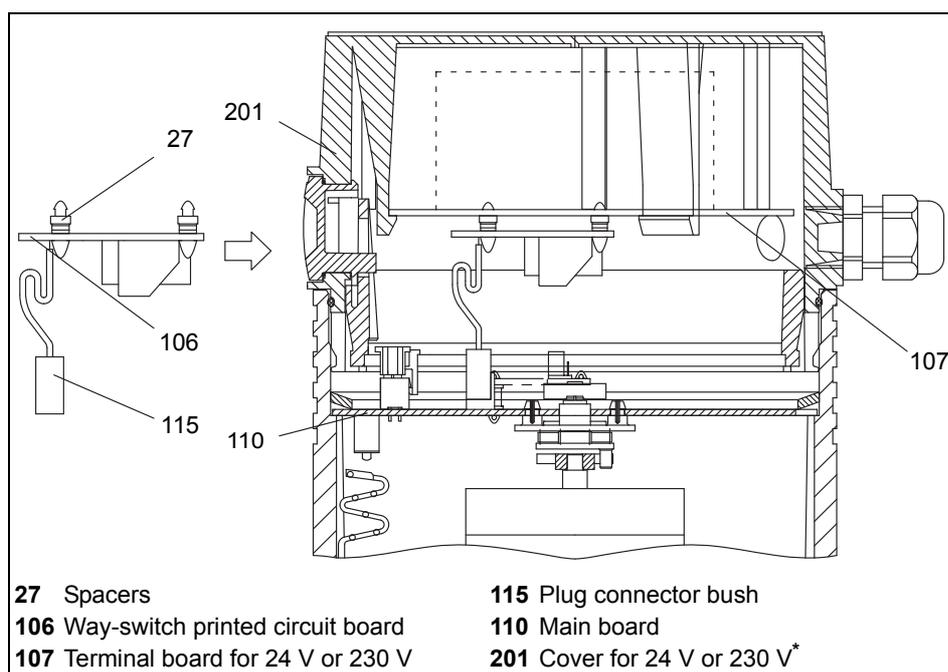
**diagram 10** Installation of the way-switch printed circuit board in the cover
