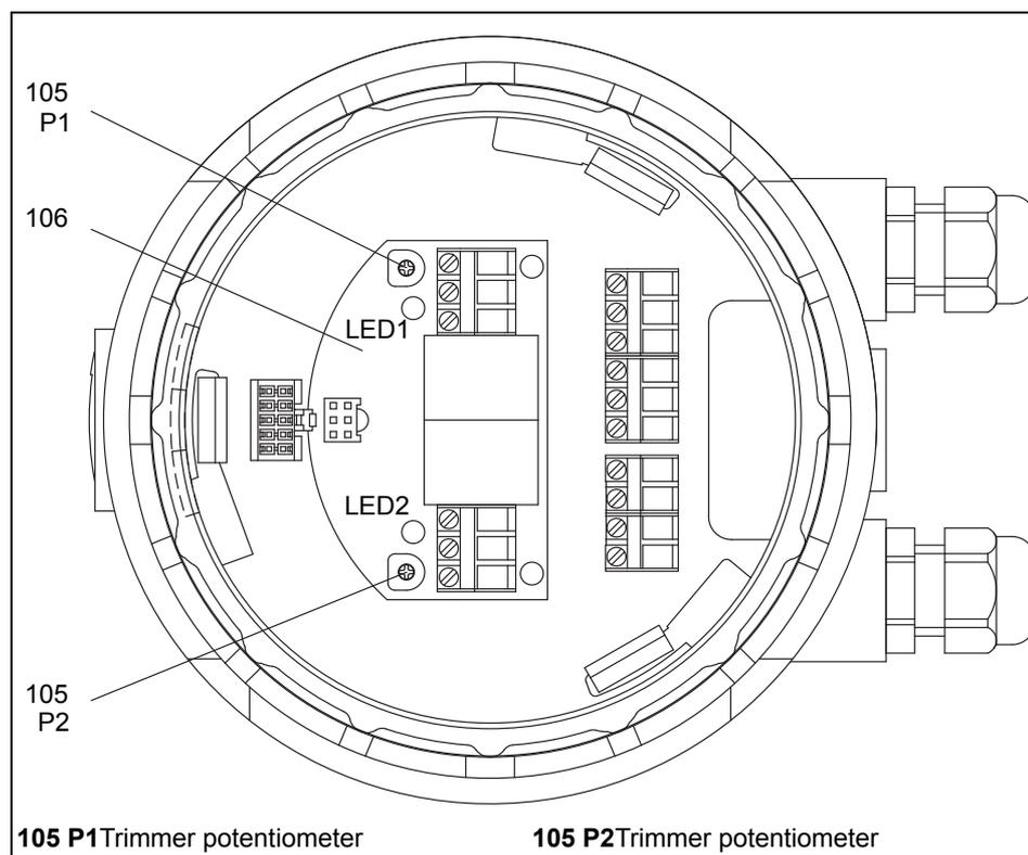
**diagram 18** Way-switch printed circuit board in cover
