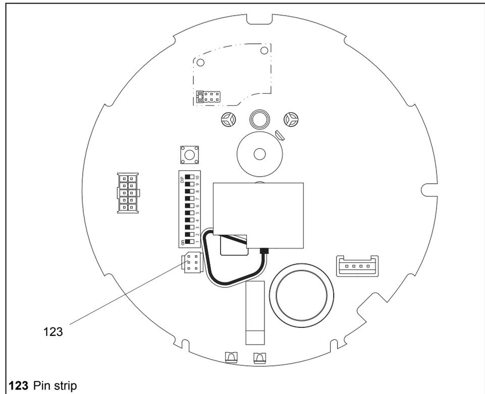
**diagram 11** Pin strip for way-switch printed circuit board on the motherboard
