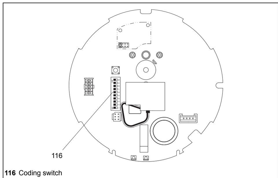
**diagram 14** Printed circuit board cover and coding switches
