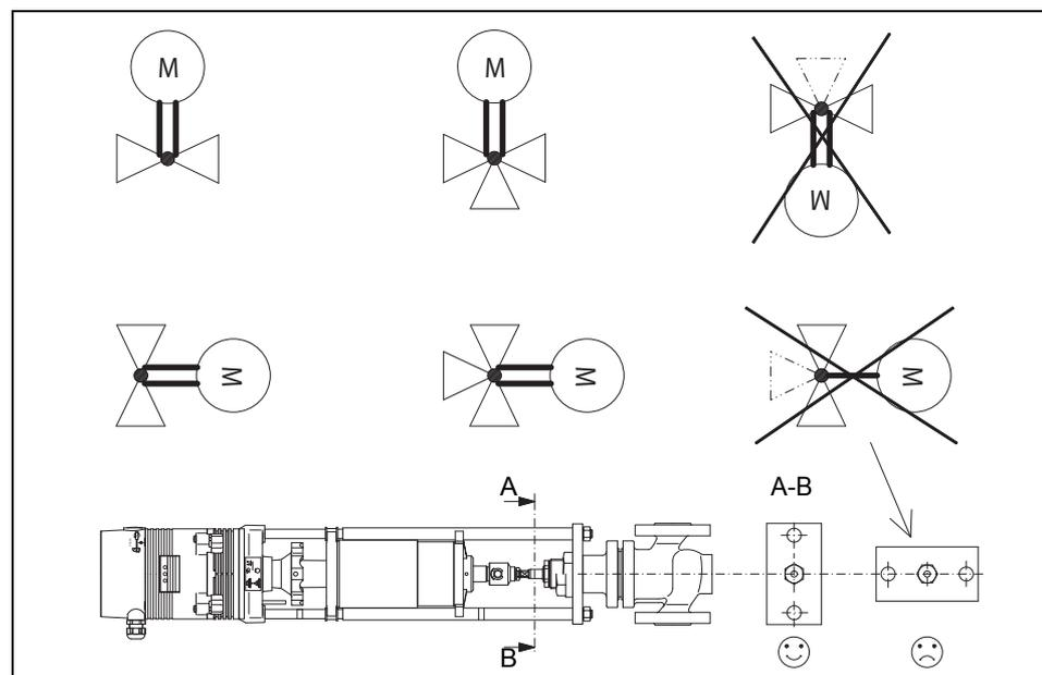
**diagram 5** Assembly positions for linear actuator and valve
