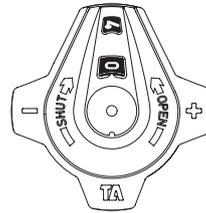
Fig. 3. Fully open valve
