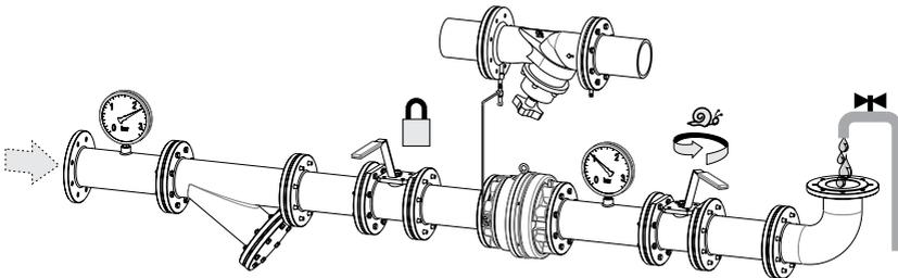
When the isolation valve on the outlet side of the DA valve is fully open and the valve is under pressure, vent the valve by using an 8 mm spanner.
