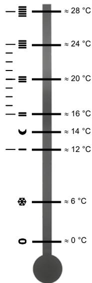
KEYMARK certified and tested according to EN 215
