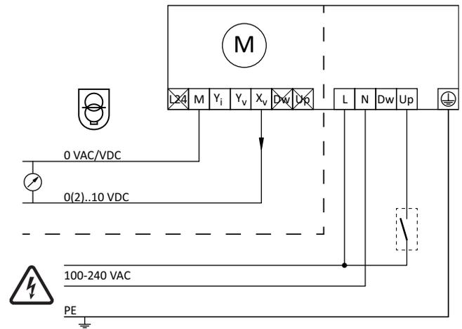
24 VAC/VDC operating only with safety transformer according to EN 61558-2-6.
