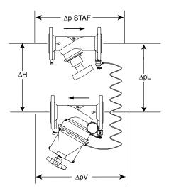
$\Delta H = \Delta p V_{_{STAF}} + \Delta p L + \Delta p V$
