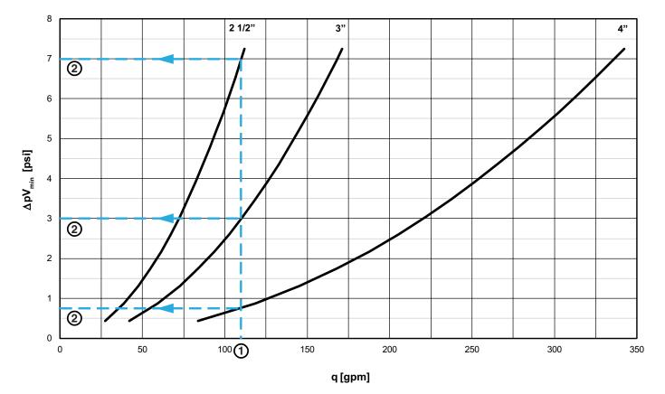
The diagram shows the lowest pressure drop required for the STAP valve to be within its working range at different flows.
