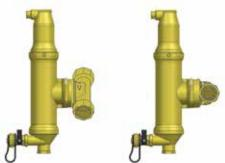
If space around the pipe on which the Turnable needs to be installed is limited, the clip that holds the separator and the rotating base together may be removed, allowing the front part to be detached. Once the threaded base is installed on the pipe, the front part can be re-attached and fixed again by re-inserting the clip from the top.
