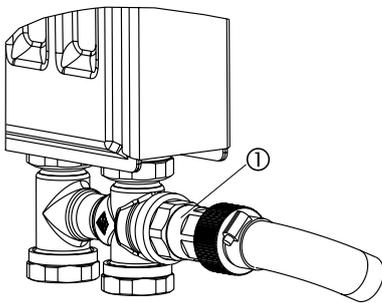
1. Drain-off facility with 1/2" hose connection
