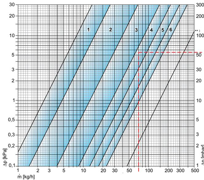
Thermostatic insert VHV8S with 8 infinitely variable presetting values
