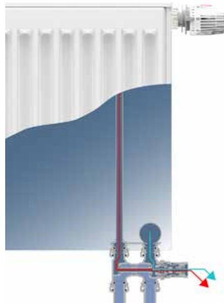
Complete drain-off of the radiator via supply and return simultaneously.
