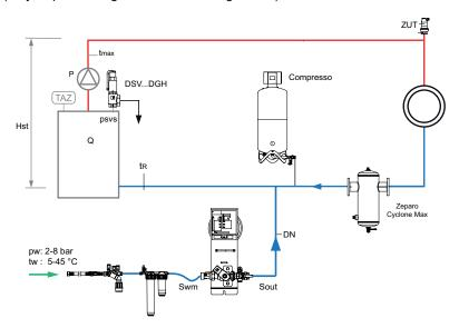
**Zeparo Cyclone Max** with magnet ZCXM for the central separation of sludge.
