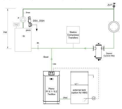
**Zeparo Cyclone Max** with magnet ZCXM for the central separation of sludge.
