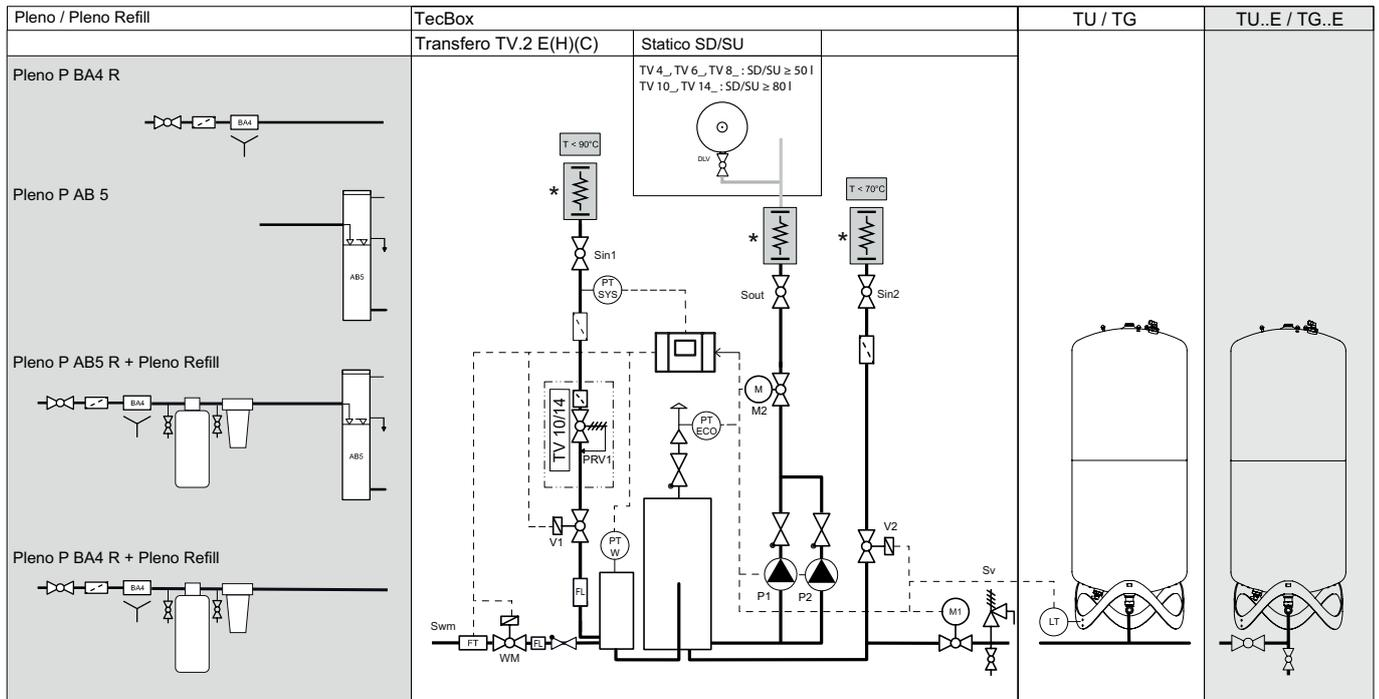
\* When connecting to rigid piping, it is essential to ensure that there is no axial, vertical or horizontal tension. The connections must not be loaded with any additional weights. Maximum tightening torques must be observed where specified. If tightening torques are not specified, the state of the art for the respective connection must be observed. **A flexible connection is preferable to a rigid connection.**
