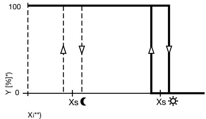
Action chart for heating operating mode with actuator in the model, closed and currentless.
