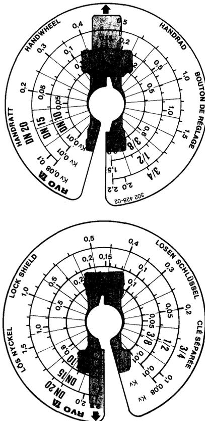
In some areas e.g. stair wells it is favourable to lock the radiator valve in a fixed pre-setting value. The locking is done as follows:
