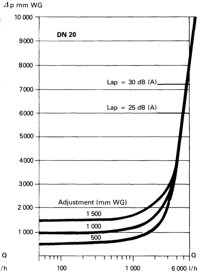
The set value can be adjusted from 500 to 1 500 mm WG (5–15 KPa).
