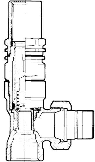
For this reason, mount a BPV valve on each branch, below the STA-D balancing valve. The essential function of the BPV valve is to maintain a constant differential pressure within the radiators.
