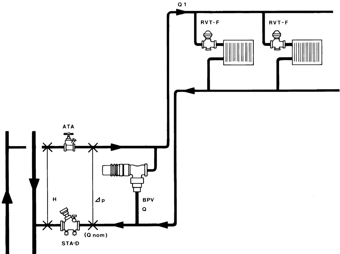
First of all it is advisable to adjust the maximum flow of each radiator to its nominal value, for instance by means of the device built in to the RVT-F and RVT-F 2S thermostatic valves.
