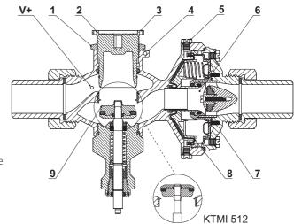
The spring force corresponds to 12, 20 or 40 kPa (Fc value) pressure difference on the diaphragm.
