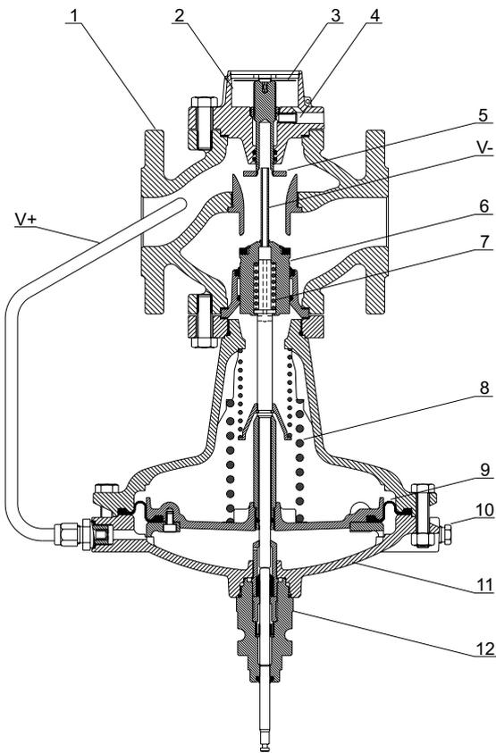
The controller consists of a valve (1), a diaphragm actuator (11) and an adapter (12) for the connection of an electromotor actuator for temperature control. The diaphragm actuator and electromotor actuator act parallelly to the valve, totally independent one from the other.
