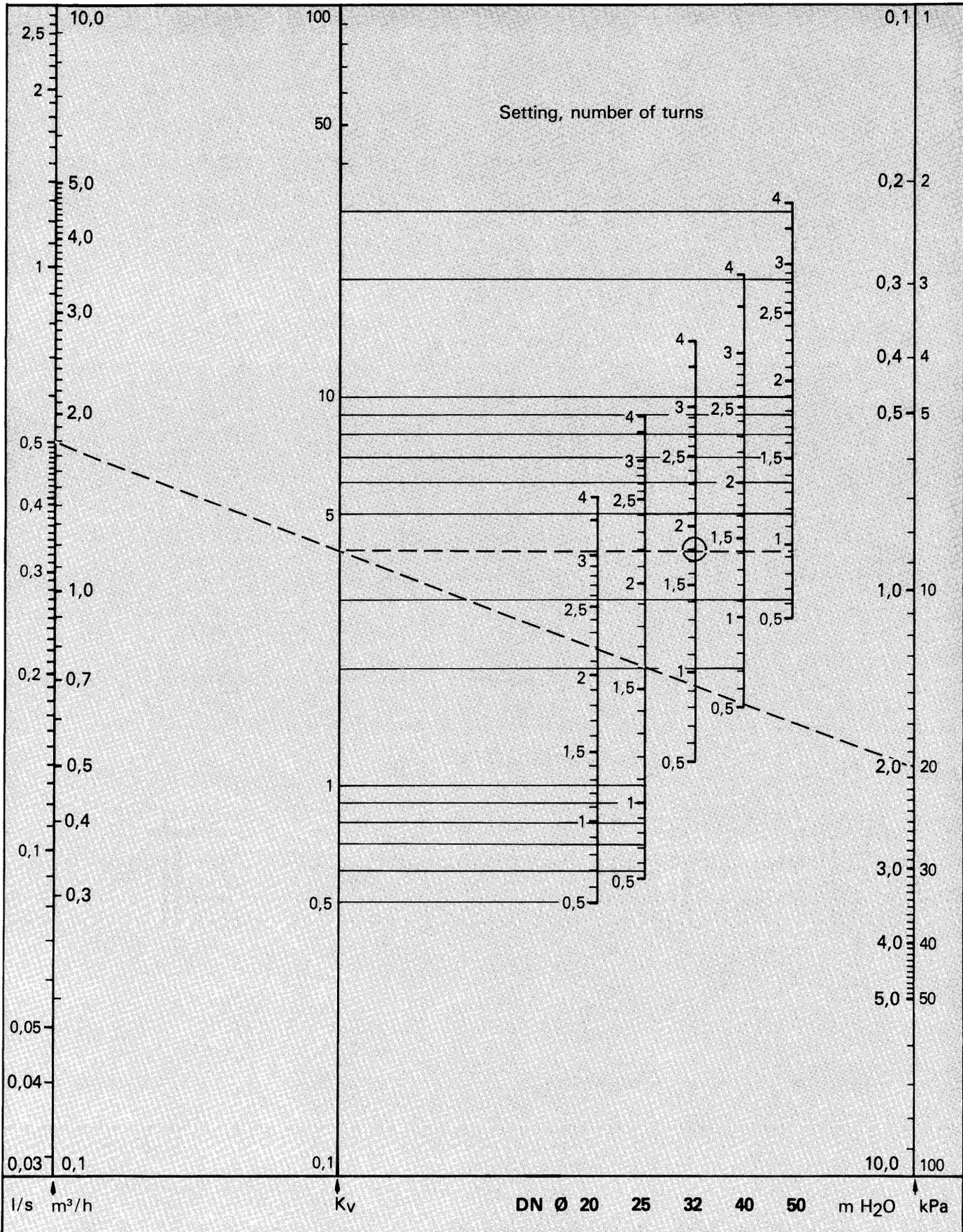
This graph shows the pressure drop over the pressure test points of the valve.
