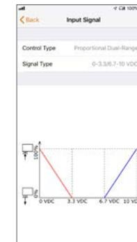
Dual-range input signal for heating-cooling changeover
