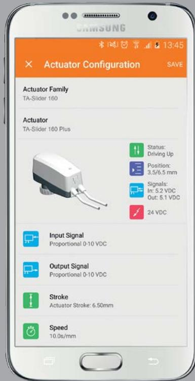
TA-Dongle enables interface between actuator and smartphone using Bluetooth communication
