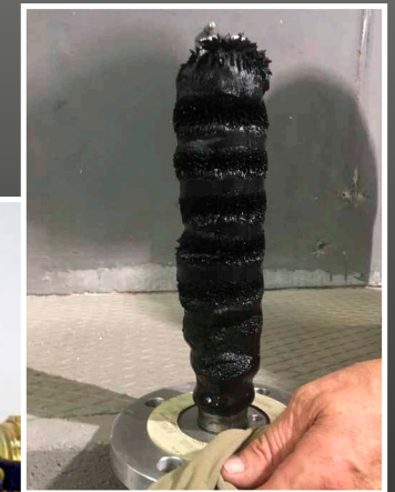
Ferro Cleaner magnet after 1 year of operation
