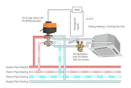
Changeover solution with three control signals and Fan-coil Terminal Unit
