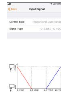
Dual-range input signal for heating-cooling changeover
