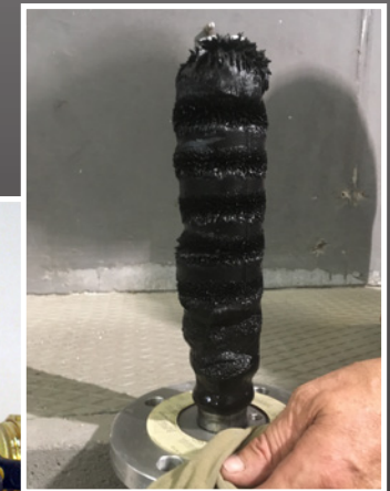
Ferro Cleaner magnet after 1 year of operation
