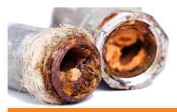
Oxygen in the system reacts with metal components leading to rust built up that clogs pipes and significantly reduces efficiency and durability of equipment.
